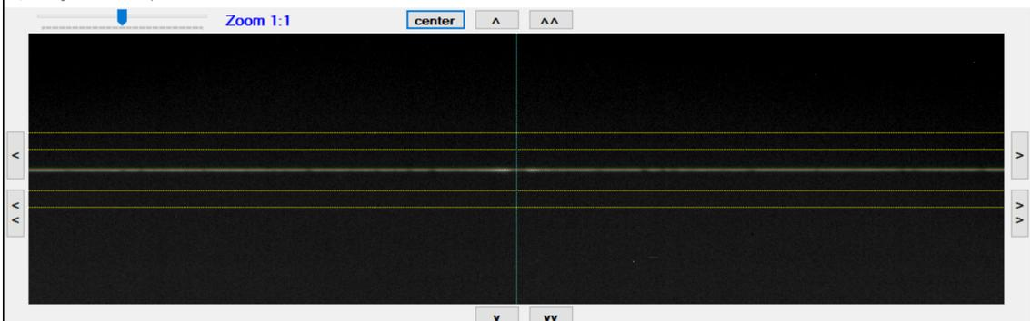
The software scans the upper and the lower background stripe and calculate an average of it (blue curve in the example). A polynomial with grade 5 is the correction curve (green curve in the example). The correction is a subtraction of the scanned spectrum minus the correction curve.
