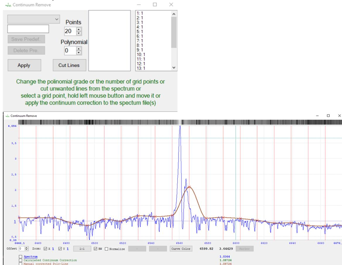
The continuum remove feature is very similar to the instrument response correction. You can cut lines, edit point, etc.
