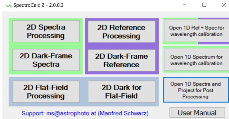
**2D Spectra Processing:** load 2D spectra for 2D-calibration, scanning and aligning
