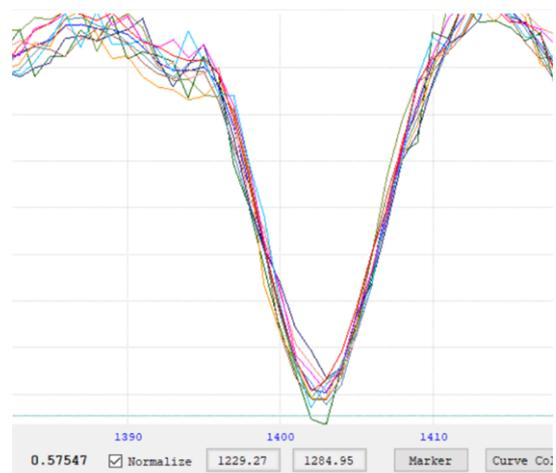
In this example, I have aligned with the spectra lines. The graphic of the aligned references shows that one reference image is completely wrong aligned. For some reasons (maybe a mechanical problem), this image was shifted against the others.
