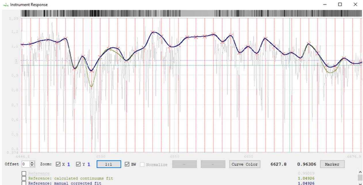
Select “Show Result” and you will see a grey curve as original spectrum, a green curve as reference spectrum, an orange curve as instrument response curve (continuum shape of spectrum divided by continuum shape of reference) and the pink shape is the corrected spectrum (original spectrum divided by instrument response).
