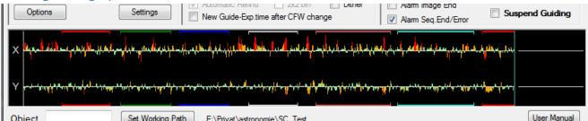
Each measured and corrected guide star deviation from the target guide star position on the chip is shown in this graph as a guiding error for X and Y axis. That means if you have a guiding speed of 8 Hz you get 8 values per second.
