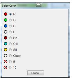
Select the required filter and the window close automatically and the filter wheel moves to the selected position.
