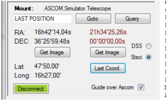
If you don't want to guide via the camera guiding port, you can check "Guide over Ascom". Attend, that most Ascom mount driver are much slower than the guiding port of the camera. Mostly it makes sense to increase the "relay aggressiveness" extremely.
