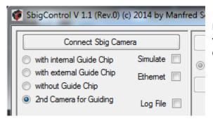
Don't forget to check "Ethernet" if you want to work with Ethernet. Ethernet is slower than USB for downloading images from the camera!
