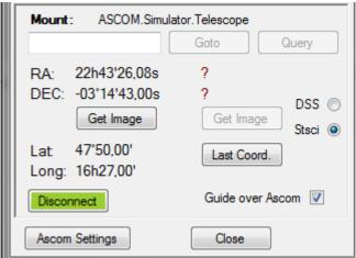
After connecting the mount driver, you can see the actual sky position in RA and DEC and the latitude and longitude which is stored in the mount.
