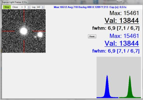
Now you get a 120 x 120 pixel sub-window of the chip (size is changeable with "Settings") and a continuous imaging in 1x1 binning. The display is zoomed to 2:1. The exposure time is automatically calculated and shown on the top line in blue (EXP.[s]: ...).
