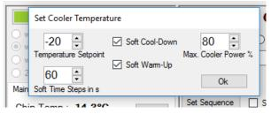
If you check "Soft Cooldown" you can set your desired target temperature and SbigControl will cool down in soft steps to avoid freezing of the chip.
